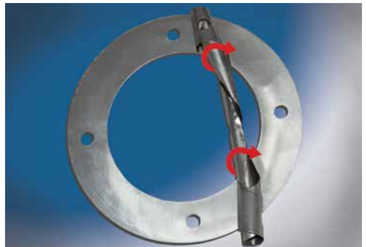
Surface Bonded Laminated Shims unwanted layer deformation
